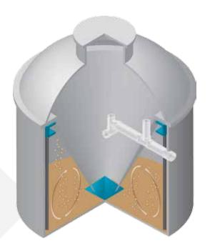
The process occurs entirely within the self-contained Whitewater ATU which is comprised of an outer mixing tank and a cone-shaped settling chamber. Raw, unsettled domestic wastewater enters directly into the mixing tank where mixing occurs through an air distribution system.
